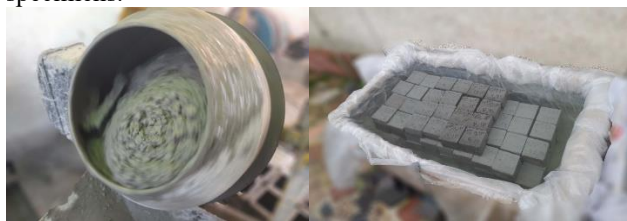
Figure 5. Concrete mix preparation and specimen curing procedures
