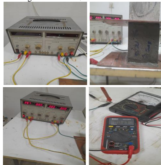
Figure 11. Specimen configuration for electrical resistivity measurement
