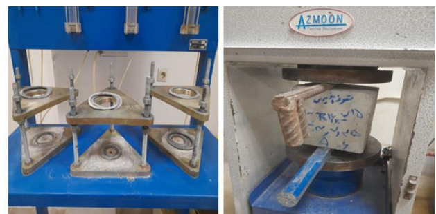
Figure 13. Specimen configuration for concrete permeability test
