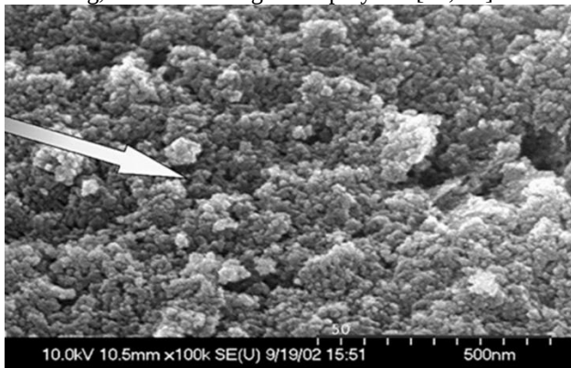
Figure 2. TEM image of a nanoparticle (“geopolymeric micelle”), 5–15 nm in size, marked by the arrow [10].
