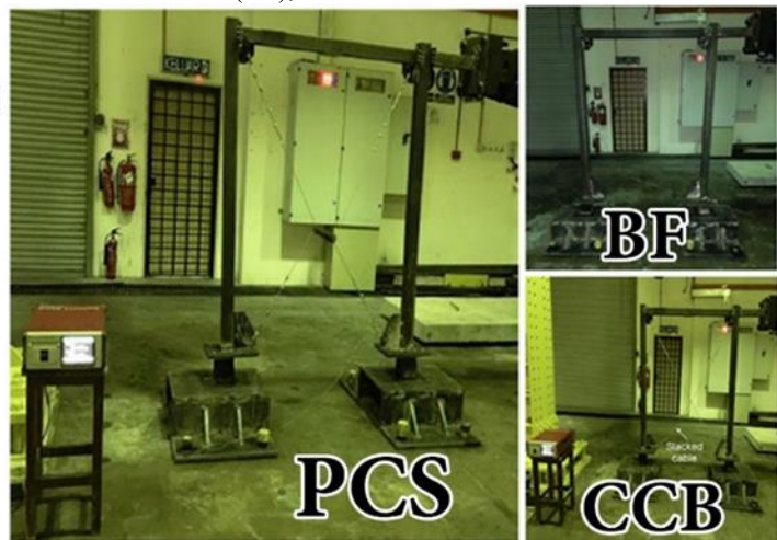
Figure 1 – Image of the three laboratory specimens and dimensional details of the cable- and spring-braced moment frame studied by Mehrabi et al. [14] under lateral cyclic loading.
