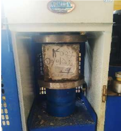
Figure 6. Compressive strength test on cubic sample
