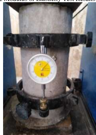
Fig. 4. Concrete Deformation in the Modulus of Elasticity Test 21 °C
