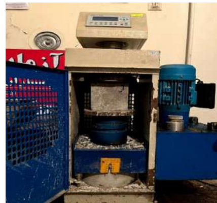
Figure 5: Jack for compressive strength testing
