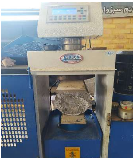
Figure 8. Testing the tensile strength of the cylindrical sample
