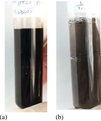
Figure 4. Dispersion of oxidized carbon nanotubes with PEG/PCE (a) solution containing MWCNTCOOH and PEG/PCE two months after ultrasonication (b) solution containing MWCNTCOOH and PEG/PCE two months after ultrasonication in a diluted form to better observe the dispersion.
