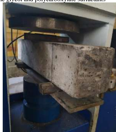
Figure 10. Flexural strength test of prismatic beam
