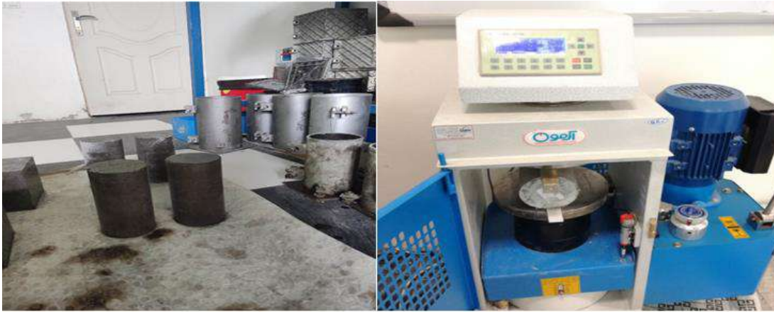
Figure 9: Cylindrical samples after being taken out of the pond and tested for tensile strength.
