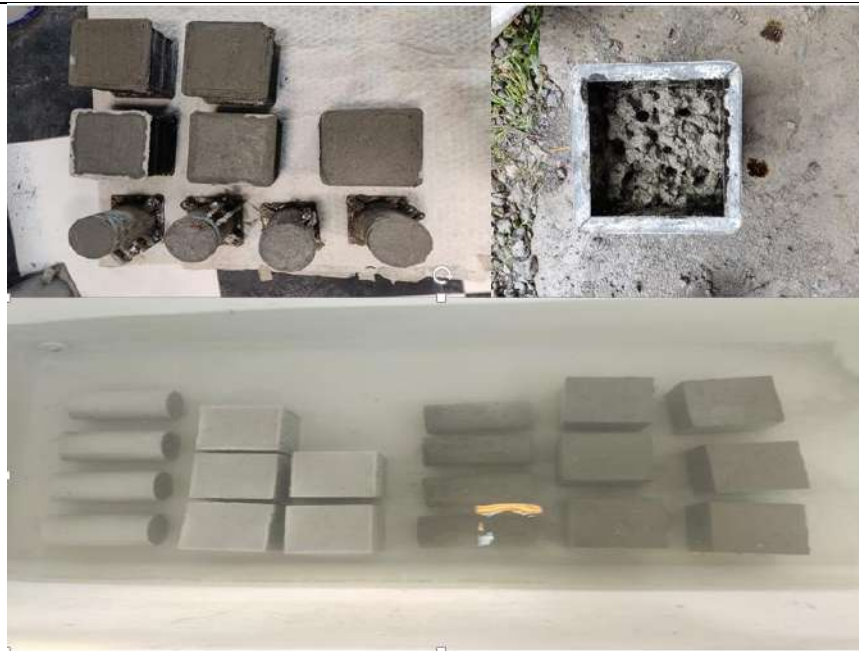
Figure 6: The process of making and processing samples.
