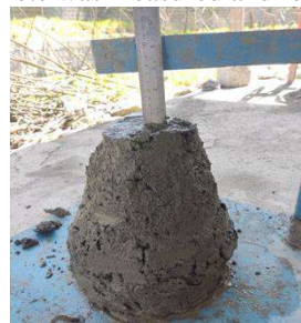
Figure 7: Concrete slump test
