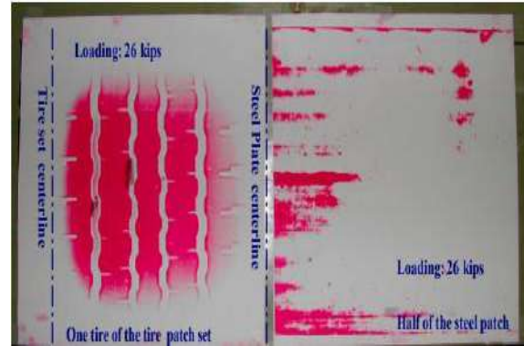
Fig. 8. Normal Stress Distributions of a truck tire and a steel plate using pressure film sensor [1]
