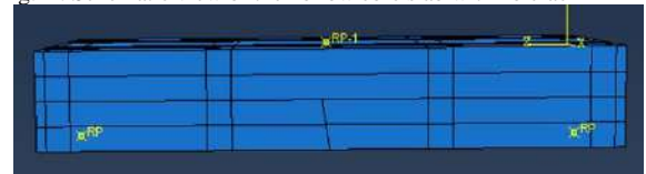
Fig. 2. Schematic view of the hollow core slab with flexural crack
