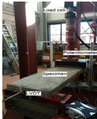
Figure 2. Boundary and loading conditions of the experimental test setup
