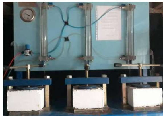
Fig. 10. Water Permeability Test in Concrete
