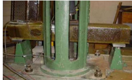
Fig.9 .How to apply force in the laboratory [3]
