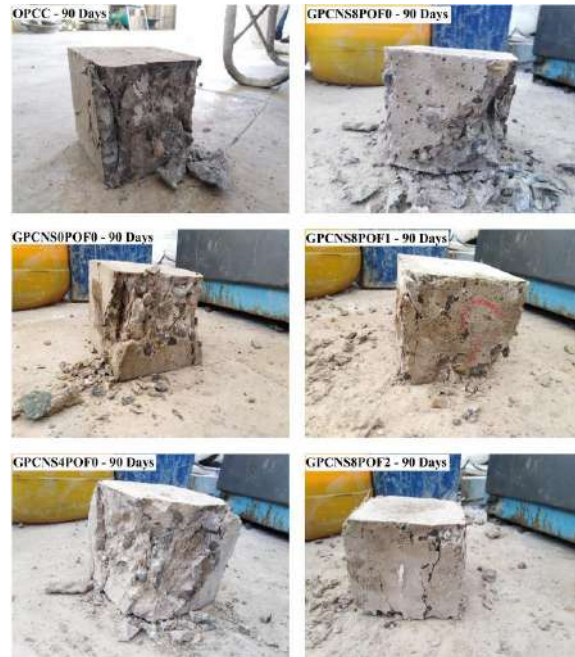
Fig. 3. Concrete Sample in Compressive Strength Test
