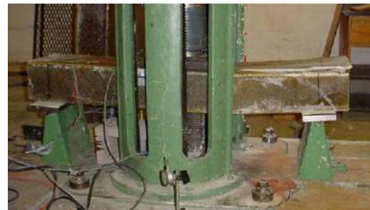
Fig.10. Separation of the upper surface from the core of the beam under load in the laboratory [3]
