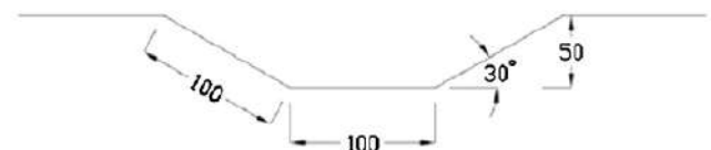
Figure (3) dimensions and wave geometry in corrugated steel shear wall [21]
