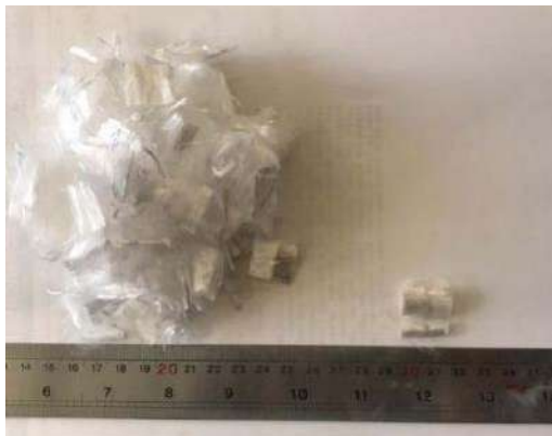
Figure 2- Polypropylene fibers used in this research
