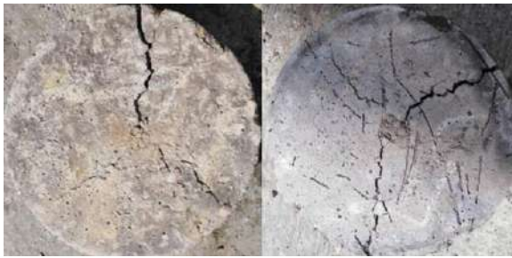
Fig. 5. Pattern of fracture of specimens in impact test
