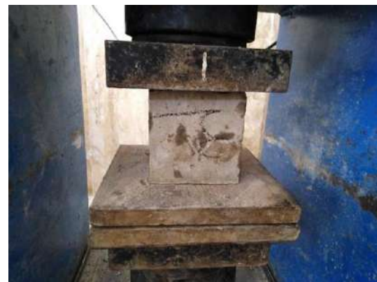
Fig. 3. Concrete sample in compressive strength test
