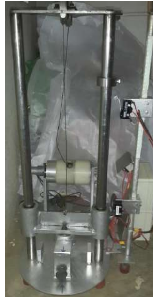
Figure 4. A device for determining impact resistance based on ACI 544
