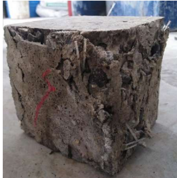
Figure 3. Concrete specimen after compressive strength test
