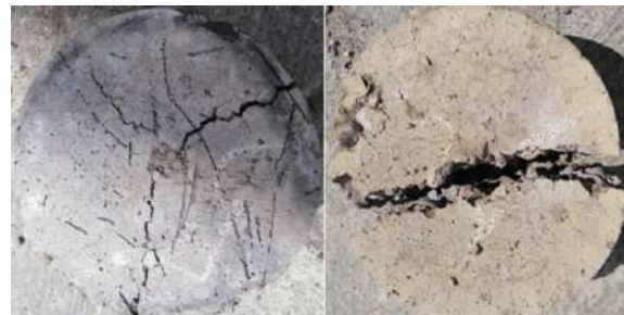
Figure 7. Concrete specimen after impact strength test
