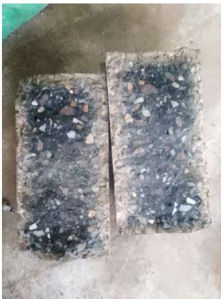
Figure 5. Concrete specimen after tensile strength test
