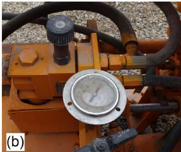
Figure5: a) Helical piles grouting operation b) Grouting pump
