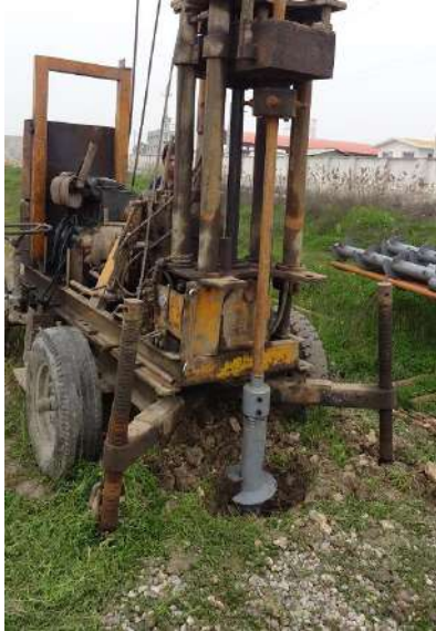
Figure 3: Helical pile installation equipment
