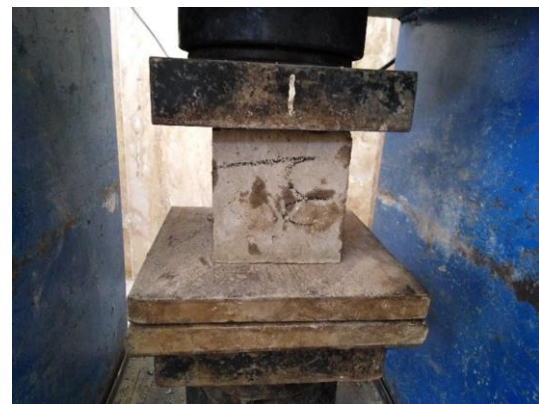
Fig. 3. Concrete sample in compressive strength test
