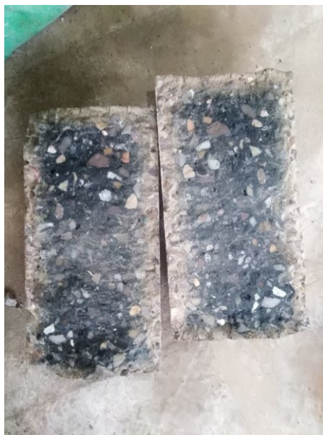
Figure 5. Concrete specimen after tensile strength test
