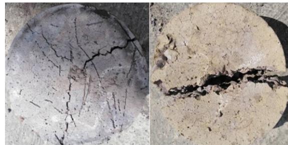
Figure 7. Concrete specimen after impact strength test
