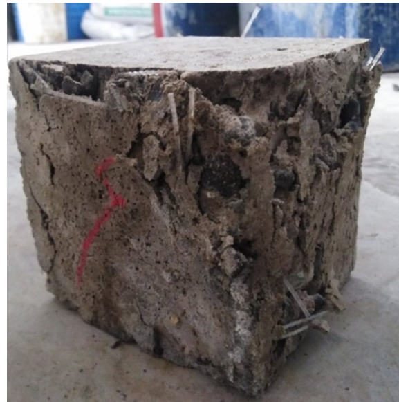
Figure. 3. Concrete specimen after compressive strength test
