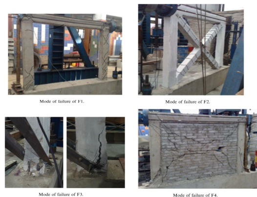
Fig. 14. Modes of failure [2]
