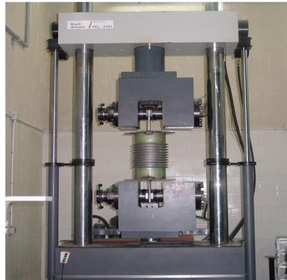
Fig. 3. Experimental test setup using uni-axial testing machine
