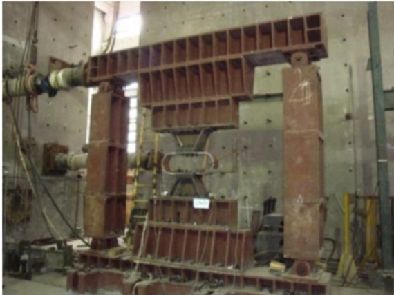
Fig. 3. Test setup of annular metal damper.
