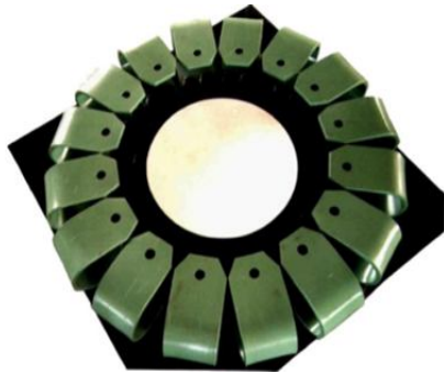
Figure 9: the U-shaped biaxial yielding steel damper with a circular arrangement
