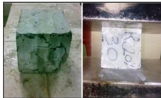
Figure 5 - Sample containing 20% crude rubber after rupture
