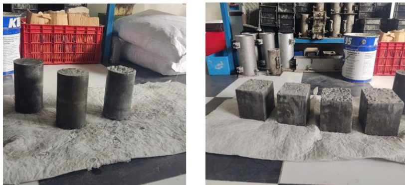
Figure 5: Cubic and cylindrical samples of control concrete
