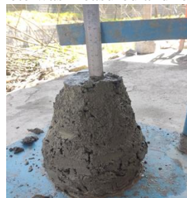
Figure 7: Concrete slump test
