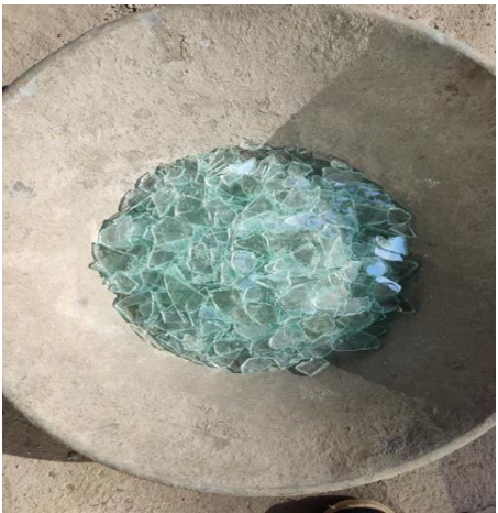
Figure 4: Appearance of used glass shards.
