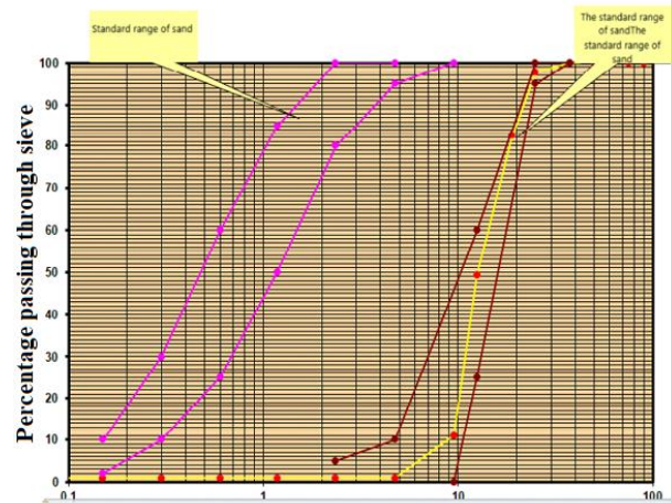
Figure 1: Gravel grading chart compared to ASTM limits
