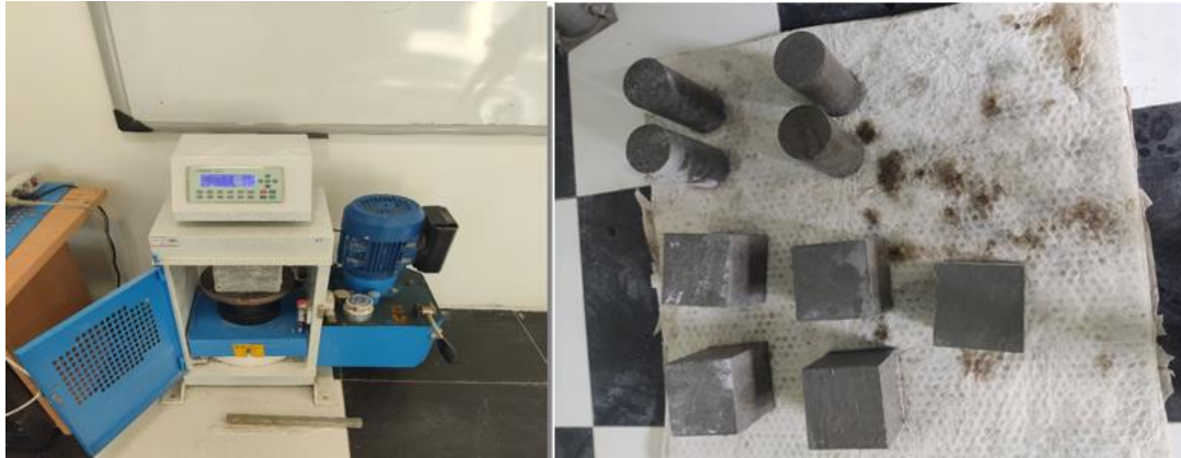
Figure 8: Cube samples after being taken out of the pond and tested for compressive strength
