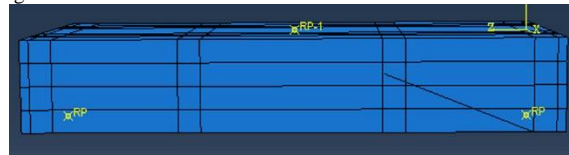
Fig. 4. Schematic view of the hollow core slab with shear crack
