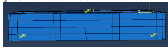
Fig. 2. Schematic view of the hollow core slab with flexural crack
