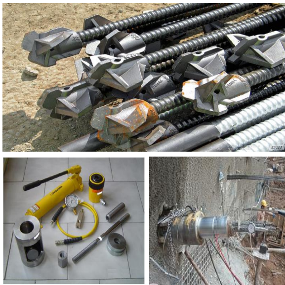
Fig 9. Hydraulic jack and the equipment of stretching the strand in anchorage method
